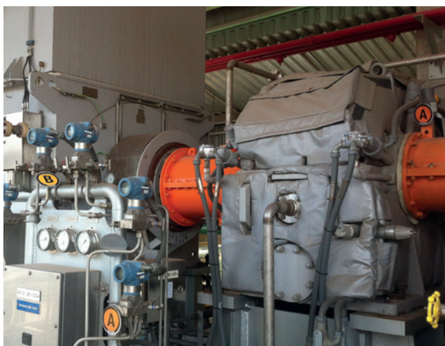
Figure 3. Propylene refrigerant compressor (left), charge gas compressor (right).
