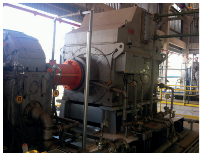
Figure 3. Propylene refrigerant compressor (left), charge gas compressor (right).
