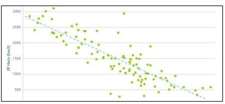
M & T diagram for natural gas consumption in correlation with external temperature; Daily level
