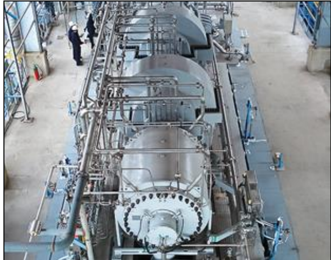
Figure 1: Cracked Gas Compressor (Source: Hydrocarbon Processing)
