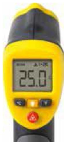
Figure 2—P1: Infrared thermometer, temperature measurement in one spot (FLIR brand on the left, FLUKE brand on the right).
