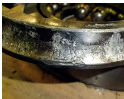
Figure 7. Condition of damaged DE motor bearings when reactor was disassembled after shutdown. Left: Outer race. Middle: Inner race. Right: Rolling elements. Both sets of the DE motor bearings were equally affected in this case (only one set shown), which is a much more severe situation than that shown in Case 1 (Figure 4).
