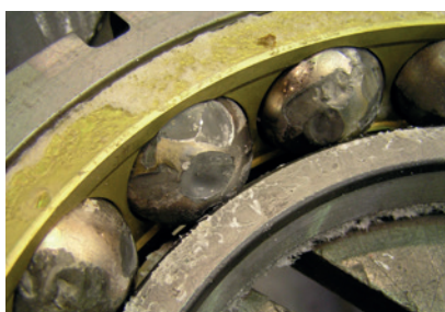
Figure 4. Condition of damaged DE motor bearings when reactor was disassembled after shutdown. Although the damage looks quite severe, only one set of the bearings was affected.
