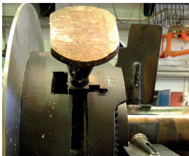
Figure 10. Condition of the middle bearing when the reactor mixer was disassembled after shutdown. Damaged bearing (right) caused by polymer that entered the damaged bearing housing and hardened. The fractured bearing housing is shown on the left.
