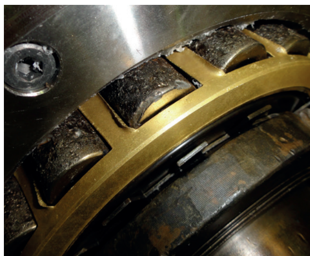
Figure 10. Condition of the middle bearing when the reactor mixer was disassembled after shutdown. Damaged bearing (right) caused by polymer that entered the damaged bearing housing and hardened. The fractured bearing housing is shown on the left.
