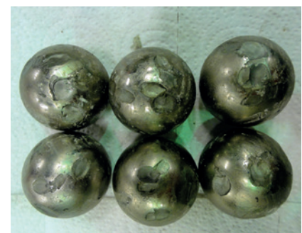
Figure 7. Condition of damaged DE motor bearings when reactor was disassembled after shutdown. Left: Outer race. Middle: Inner race. Right: Rolling elements. Both sets of the DE motor bearings were equally affected in this case (only one set shown), which is a much more severe situation than that shown in Case 1 (Figure 4).
