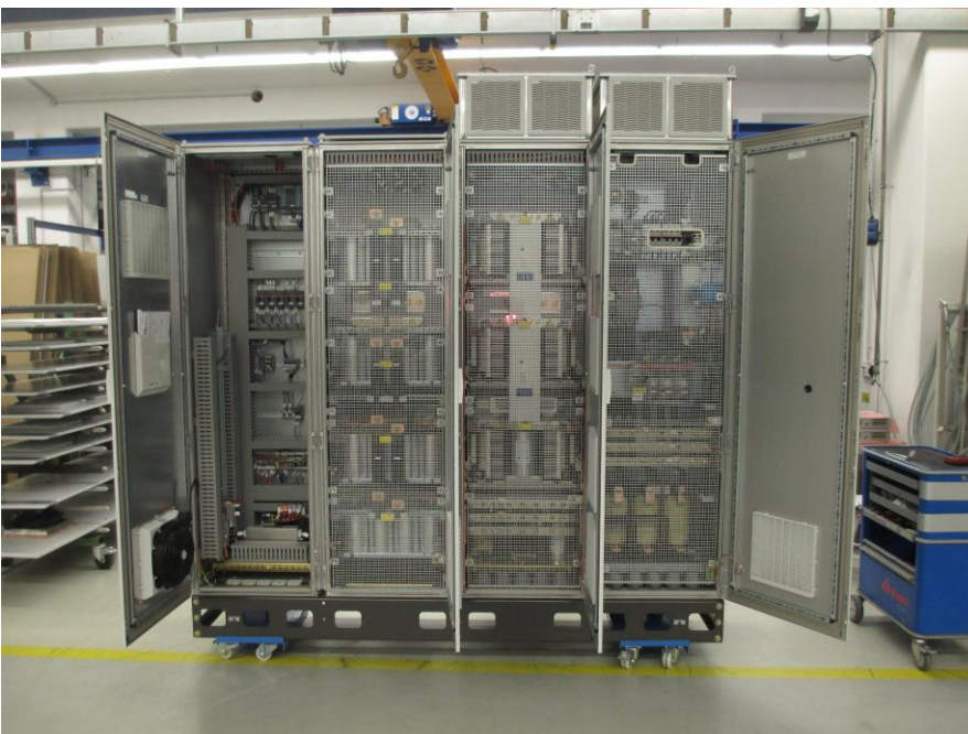
Modular designed frequency converter of Knorr-Bremse PowerTech with DC bus and active front end for test rigs applications in the railway industry.
