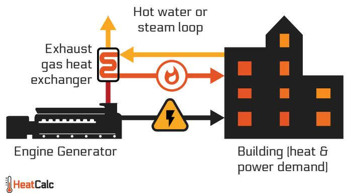
It's important to make sure there is room for a heat exchanger to extract the heat from the exhaust and transfer it to pressurized water, steam, or for use in another device.
