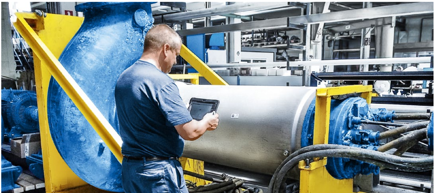
Quick, straightforward access to pump data with KSB Equipment Management: data accessed via a QR code on the pump set is displayed on a tablet browser.
